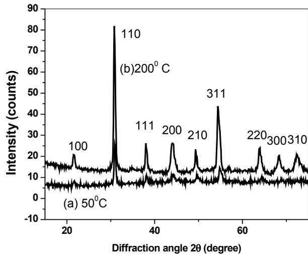
Fig.(2) XRD diffraction pattern of the PZT-5A at: (a) 50 C<sup>0</sup> and (b) 200 C<sup>0</sup>
