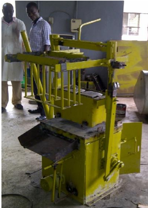
Picture of the Fabricated Double Mould Vibration Compactor Block Moulding Machine
