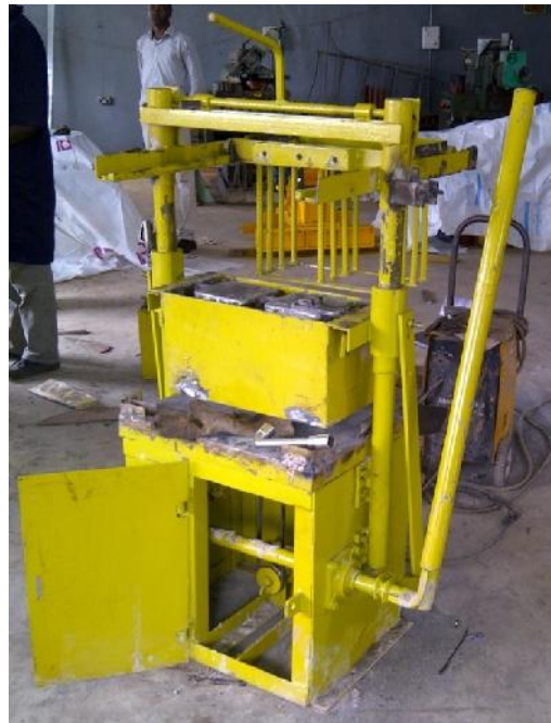
Pictures showing different side views of the Double Mould Vibration Compactor Block Moulding Machine(during fabrication)
