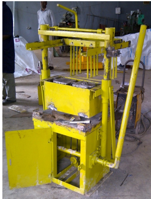
Figure 7: Pictures showing different side views of the Double Mould Vibration Compactor Block Moulding Machine(during fabrication)
