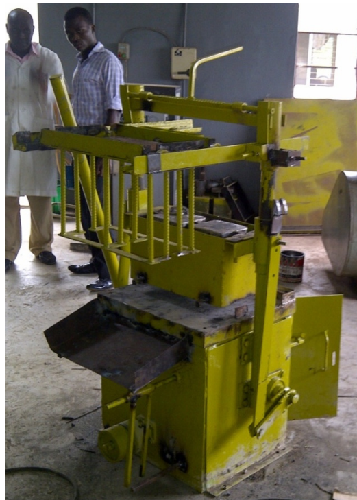
Figure 6: Picture of the Fabricated Double Mould Vibration Compactor Block Moulding Machine
