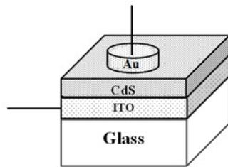
54 **Fig.1 Schematic diagram of fabricated Au/nanoCdSSchottky device**
