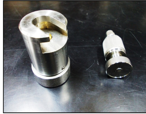
Figure 1: (a) Schematic probe and sample (b) Agilent 85070B dielectric probe (right) and the shorting block (left)
