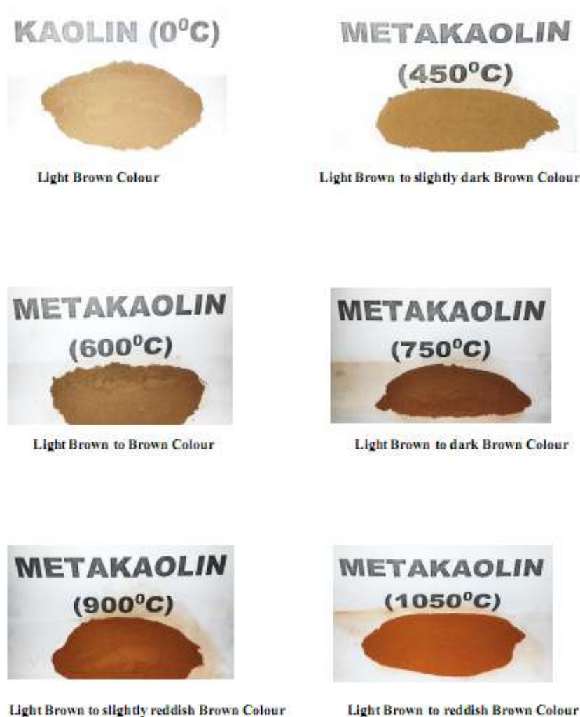
Figure 1: Kaolin Samples with different calcination temperature
