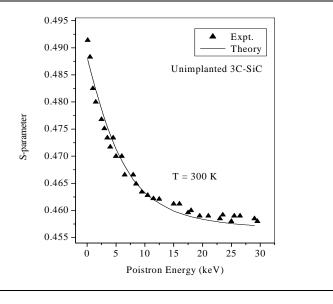
**Figure 1.** Comparison of the calculated S-parameter in unimplanted 3C-SiC as a function of incident positron energy with the experimental results of Uedono et al. [25].
