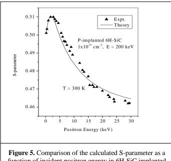
function of incident positron energy in 6H-SiC implanted by 200 keV P<sup>+</sup> ion at a dose of  $1 \times 10^{15}$  cm<sup>-2</sup> with the experimental results of Uedono et al. [11].
